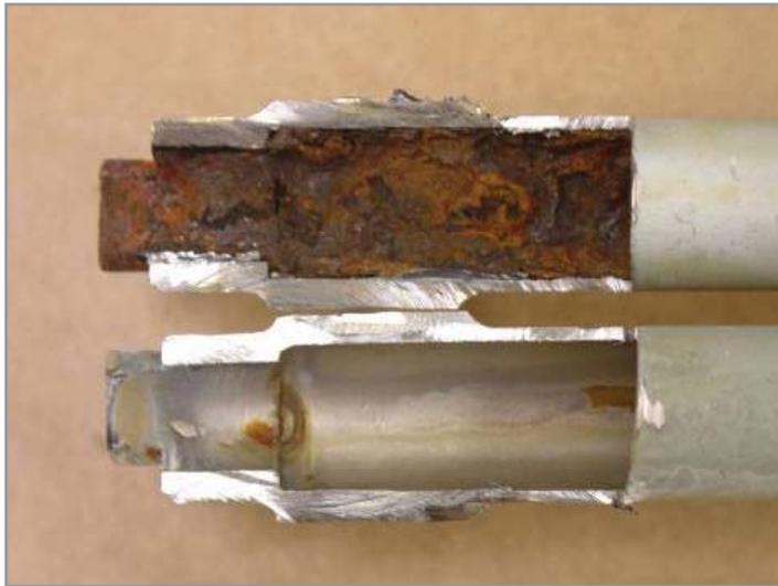
Corrosion on aircrew escape system structural tubes
